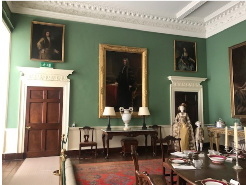
Figure 22 Dining Room, Door behind costumes (on the right) false to balance symmetry of door to Butler's Pantry (on left of image)
